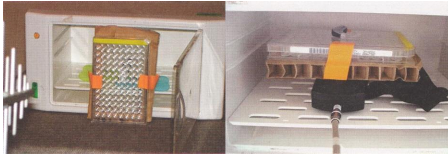
Figure 1: Defined experiment arrangement for measurement of the radiation behavior (distant field on the left) and the specific absorption rate (SAR) in the near field (right). The hearing aid is located in the left picture behind the culture dish, the second hearing aid is located in the right picture under the culture dish directly on the dosimeter.
