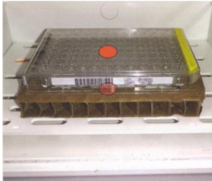
Figure 2 (above): Arrangement of the 96-hole culture plate in the incubator for the cell exposure. Both red dots designate the position of both hearing aids.
